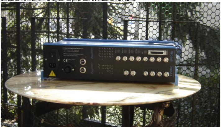
**Time - 8 to 64** synchronous channels; **very low aperture time** (minimum time between two events. (BY2K 8 channels)
