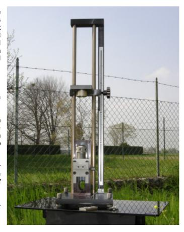
The electromagnetic locking-releasing system: is low voltage powered with built in line filters to prevent noise to/from power line
