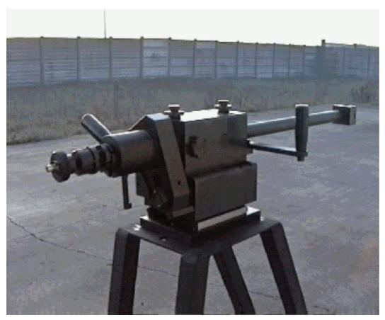
Type A rest is the standard model for the ammunition shotgun test. using 30mm diameter barrels and the with extractor mounted on the rest (this means that barrels with different chamber lenght and same caliber can share the same extractor). The pressure transducers are installed on the assembly ( the barrels have a pass through hole only ).. The length of the barrels for this support is typically 700mm. The range available calibers spans from from cal 8 C. F. to cal 12/89.
